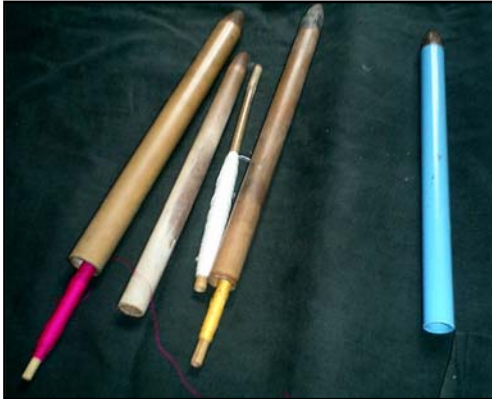
#5. Fai Sukong's first weaving tools, (left) polished bamboo shuttle bobbin case style and stick bobbins, (right) new plastic bobbin case shuttle with metal tip.
