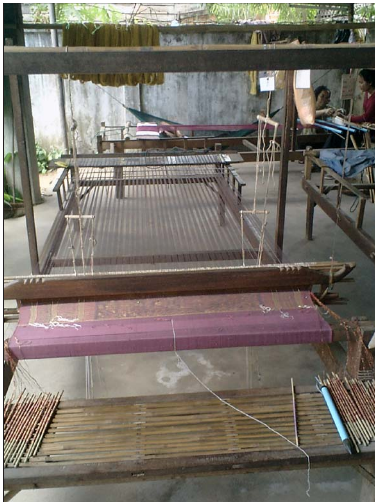
Hol weaving is in progress on a typical Cambodian loom. The weft threads have been wound on bobbins and carefully kept in the correct order on the weaver's bench.
